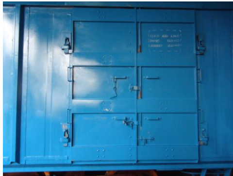
Design Iteration ( Pressed Door design- 4 hinges)-Variant-II (June'2009)
