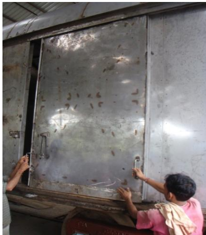
Sliding door (Pressed design): Top mounted Roller on Guide Channel (Apr'2010)
