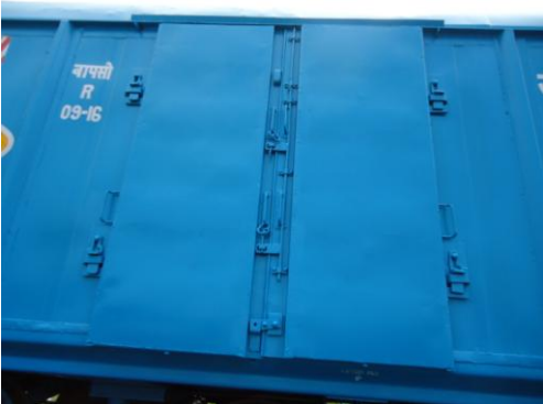
Outer view of door locking arrangement
