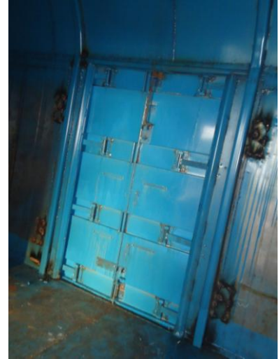
Design Iteration ( Pressed Door design- 4 hinges)-Variant-II (June'2009)
