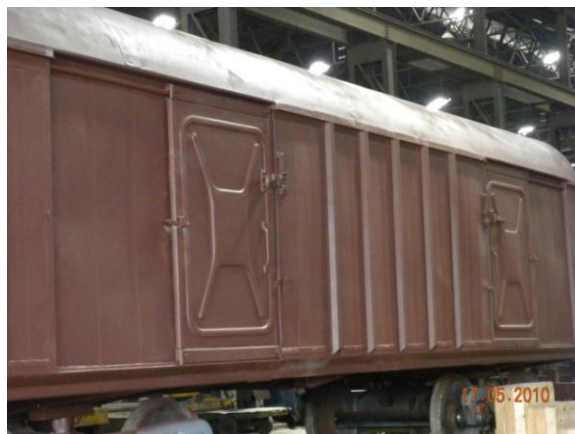
Sliding door (Pressed design): Top mounted Roller on Guide Channel (Apr'2010)
