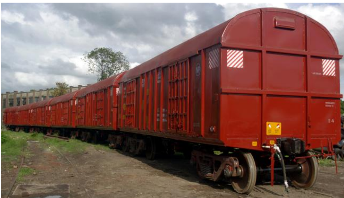
Rake of New BCNHL wagons (TWL) with 2 Part Sliding Door Wagon under operations in SCR (Wadi Division), NR (UMB Divn)
