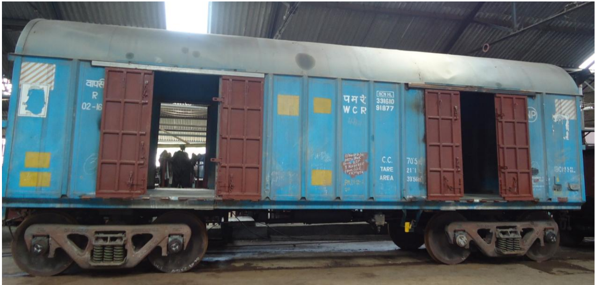
In-service Wagon No. WCR 33161091877 retrofitted with 2 part sliding door at PRTN W'shop-WR. 2 such wagons under field monitoring by GIM (Gandhidham) Depot-WR
