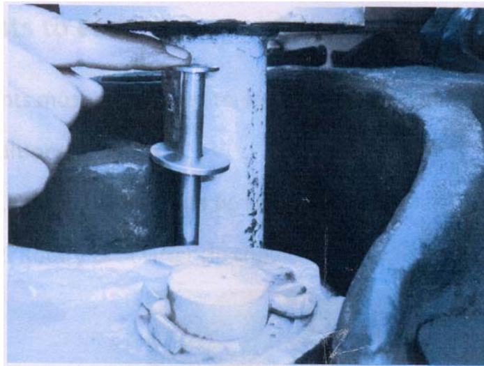
Gauge for measuring difference in height of coupler
