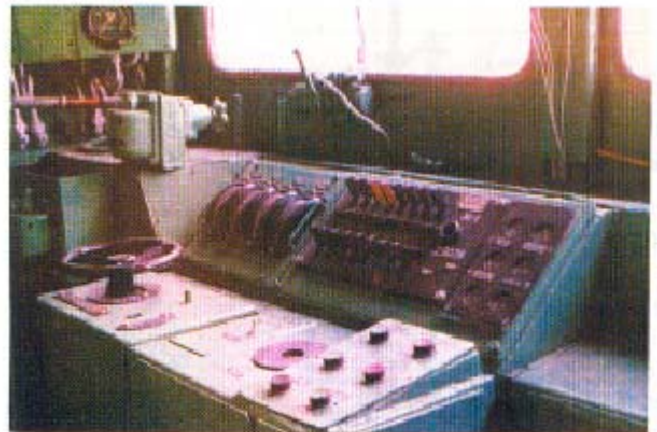
Plate 4. Driver's cab showing master Controller
