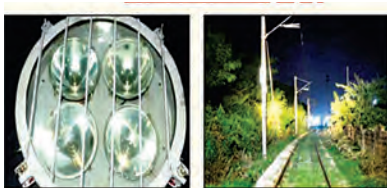
A view of 4 Beam Headlights to Improve Proper Visibility at Curvature Locations- Designed And Developed East Coast Railway
