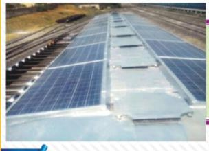
Jabalpur: Solar panels on GS coach no. 94408 (Train no.51701) have been provided for charging batteries and feeding electrical load during day time.
