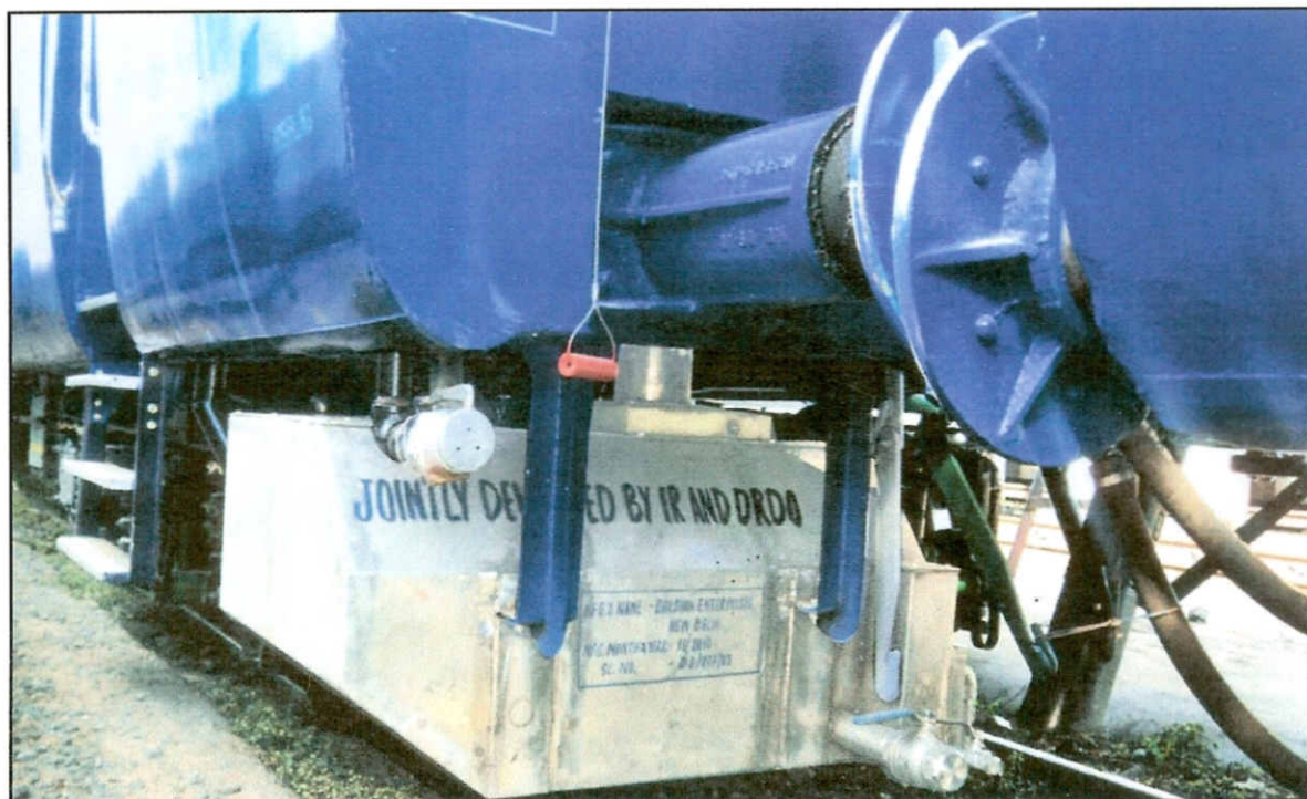
Bio-toilet (developed jointly by IR & DRDO) fitted on a coach of Gwalior-Varanasi Bundelkhand Express
