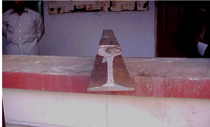
Fig.3.5.2: Fractured Rail Piece with Kidney Flaw
