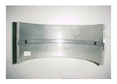
Visual examination indicates that, the bearing has several deep scoring marks & the tin flash has peeled off from about 10% of the bearing surface. There is no other damage like layer peel off or chip out.
