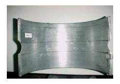
There are several deep scoring marks on the bearing surface. Otherwise, there is no evidence of peel off or chip out.
