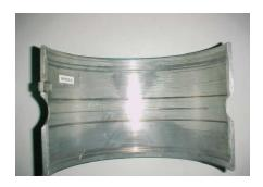
There are several very deep scoring marks on the bearing surface, besides slight exposure of the bronze in between two of such scoring marks. The tin flash also is thick. There is no evidence of layer peel off or chip out.
