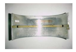
Bronze layer of this bearing is exposed in the middle in about 4"X1" area. There are several –several deep scoring marks. No evidence of layer peel off or chip
