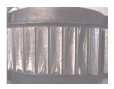
Fractured surfaces show varying degrease of progressive cracks, being around 70% in the first of the broken tooth. These cracks had started from root fillet. Almost every one intact tooth shows abnormal wear and abnormal pitting in addendum and dedendum.
