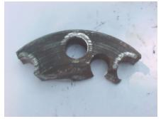
The bolt hole shown above is enlarged. Inner face of the flange is showing deep machining marks. The fractured face shows about 25% fatigue crack, about 25% final rupture and the remaining area is battered.
