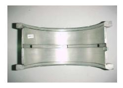
The bearing surface shows negligible distress. The bearing shows crack in the fillet of the collar .
