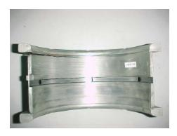
This bearing also shows crack in the fillet of the collar. There is otherwise no evidence of any damage.
