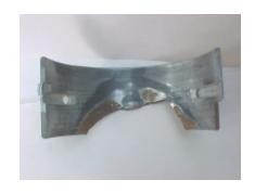
The central portion of the plated side shows biased wear in the area which had broken and separated.
