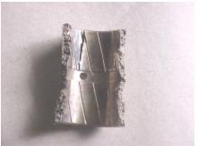
There is no evidence of any casting defect or abnormal wear. Its failure appeared to be consequential. Detailed analysis of this bush was therefore not taken up
