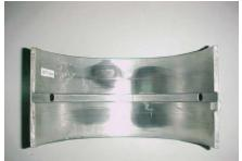
Visual examination shows that the bearing surface has blackened at four spots. This black spot is surrounded by wear marks. There is also evidence of deep scoring mark at one place and few scratch marks at places. The bearing however does not show any evidence of layer peel off or chip out.
