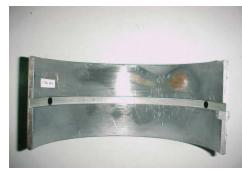
Bronze layer is exposed in about 15% of the bearing area. Steel back shows lack of proper contact with the housing. There are several shallow scoring marks. There is no evidence of any layer peel off or bearing metal chip out.
