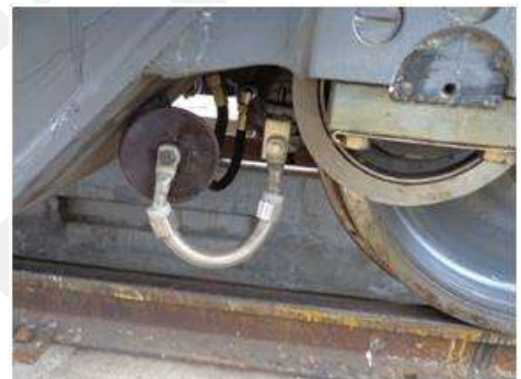
Figure 1.19 Earthing resistor assembly
