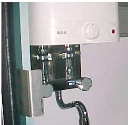
Figure 7.8 Water Boiler in Original design Coaches
